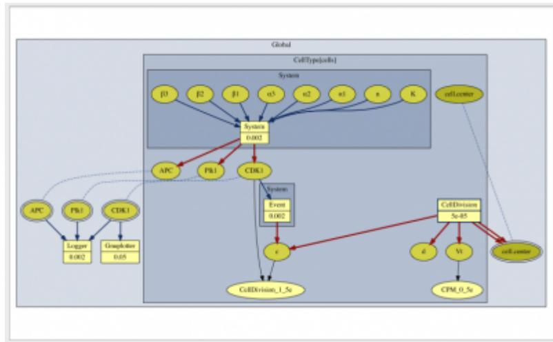
Symbol graphs show how Morpheus interprets the model. This can be used for model testing and tracing bugs.
