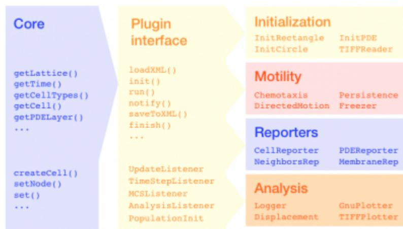
Plugin interface provides interfaces for various types of plugins.
