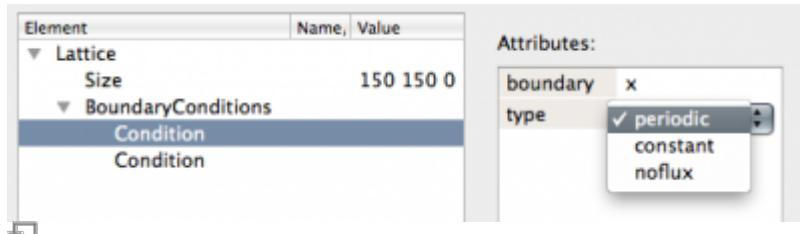
The structure of the borders is defined in Space → Lattice → BoundaryConditions.
